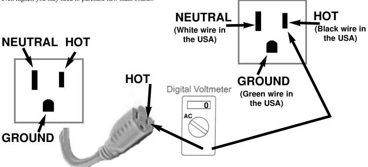
After checking the HOT to HOT above, do the same with NEUTRAL to NEUTRAL and GROUND to GROUND. As above, the difference should be no more that 3 volts, and hopefully even less.
