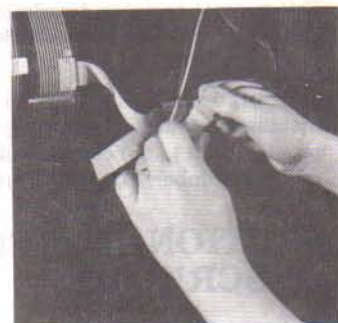
Figure 4. Attaching speaker harness
