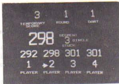
Figure 2. Stuck segment indicator display
