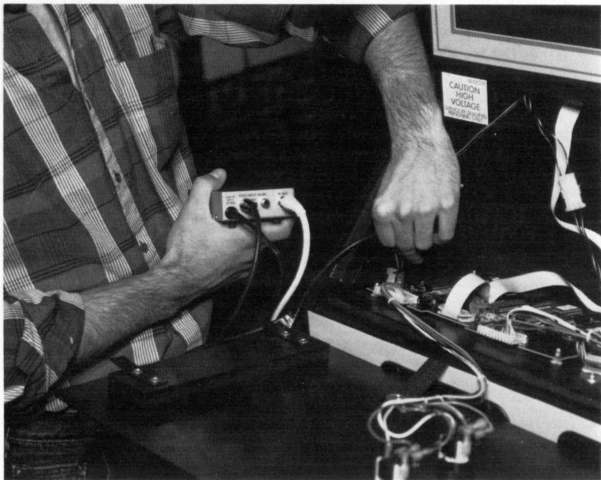
Figure 15. Hooking up a modulator for external TV
