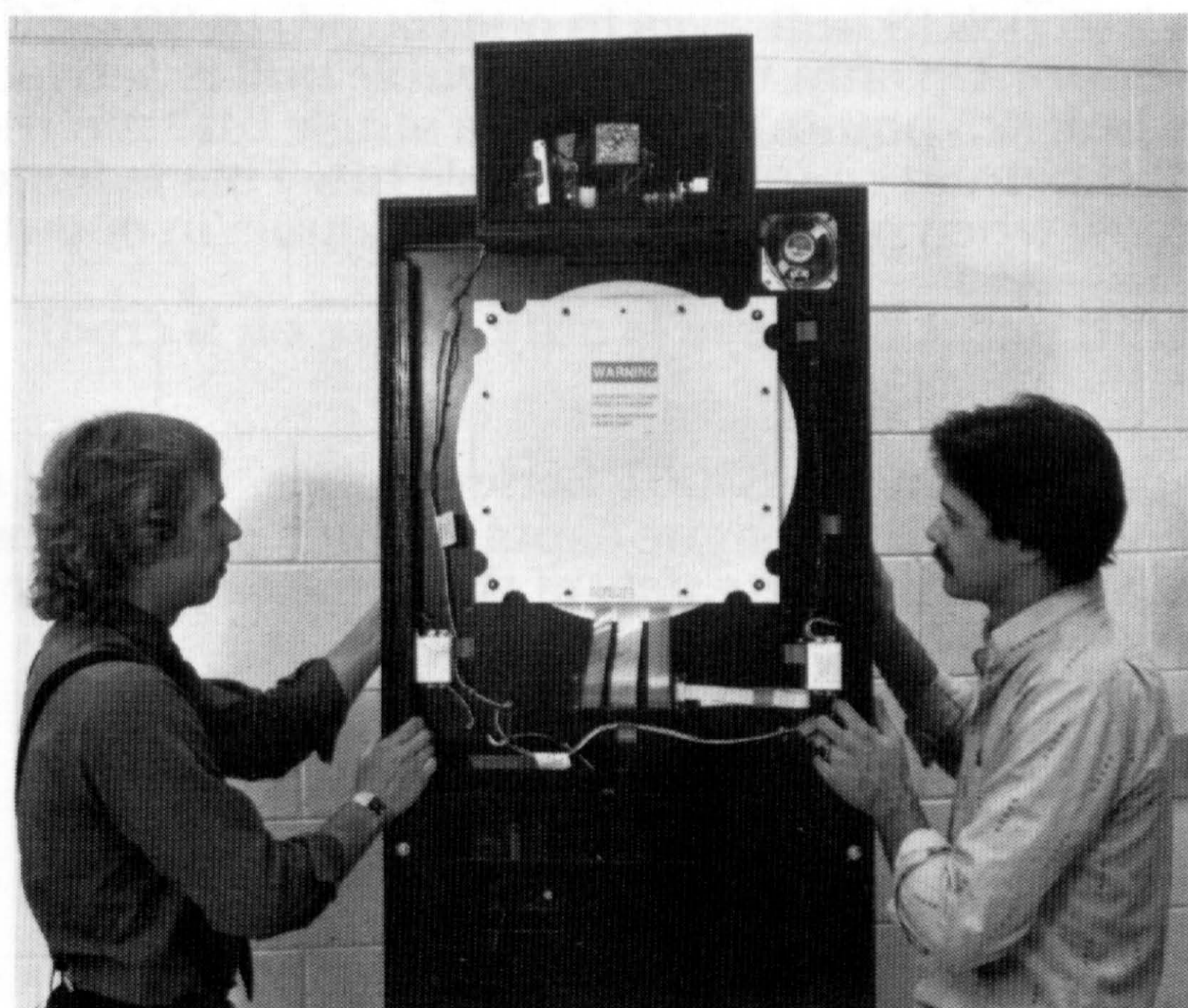
Figure 3. Attaching top assembly to base.
