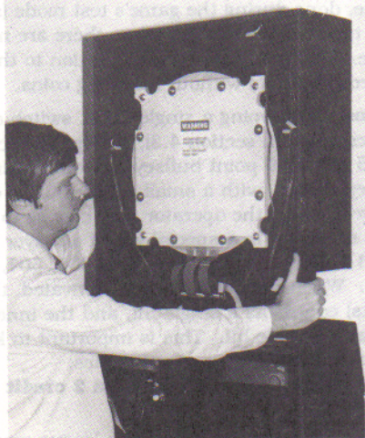
Figure 3. Attaching top assembly to base.
